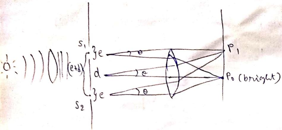
Let the light rays are passed through the double slit whose width are 'e' which are separated by a distance of 'd'. The distance from the middle points of the slits is  $(e+d)$ .
