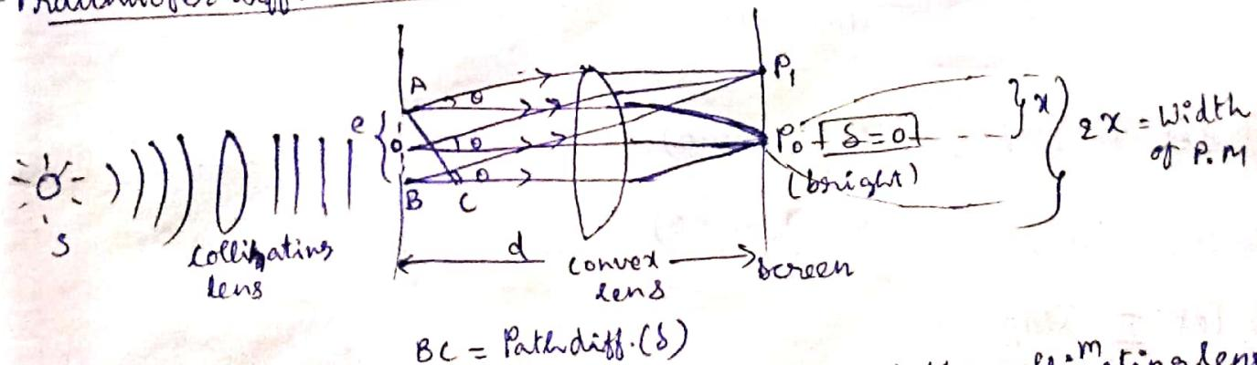
Let a monochromatic light ray is passed through the collimating lens in order to get the plane wavefronts, which passed through the slit AB of width 'e'. The diffracted light rays through the slits are focussed on the screen by means of convex lens.
