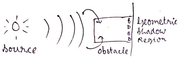
→ The phenomenon of bending of light rays around the corners of an obstacle and spreading of light waves into geometrical shadow region of an obstacle placed in a path of light is called diffraction.
