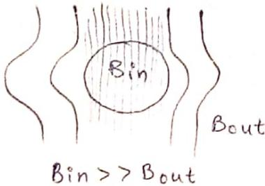
→ Above super conducting transition temperature, it behaves like a para magnetic material.
