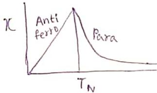
→ As the temp. increases, susceptibility increases and reaches maximum at  $T_N$  (Neel temp). Above this temp. material behaves like paramagnetic material.
