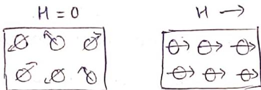
→ Since the magnetic moment is in the same direction of the applied field then intensity of magnetisation is +ve.
