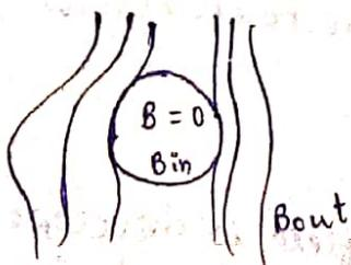
→ Above super conducting transition temperature, diamagnetic material behaves like a normal conductor.
